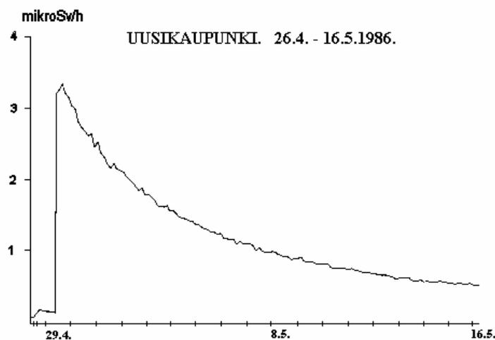
Fig. 1. Example of the effect of rain on observed external dose rates during the Chernobyl accident (Uusikaupunki, Finland).
