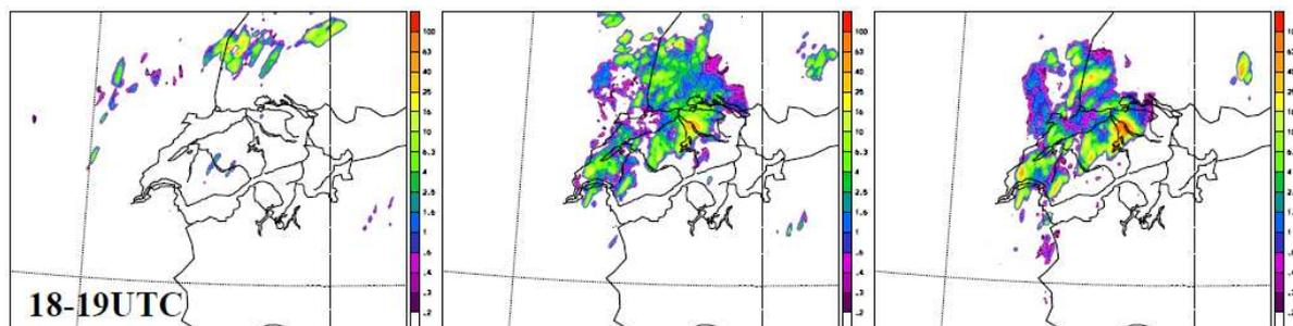
Fig. 1. Example of impact of precipitation assimilation on the 1-hour accumulated precipitation forecasts (COSMO LM model, 8 May 2003, 18-19 UTC, west of Switzerland). From the left: result without radar data, with radar data assimilated using LHN (Latent Heat Nudging) method, radar observation (Leuenberger et al., 2005).
