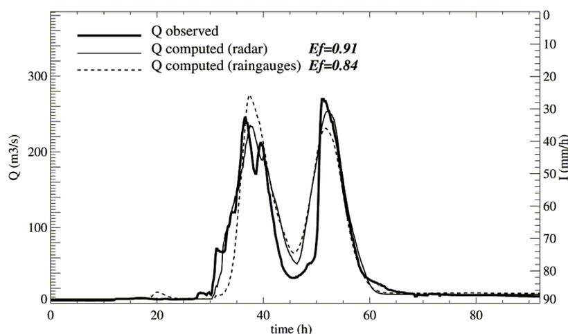
Fig. 2. Comparison of radar- and rain gauge-derived runoff simulations with observed flow (Corral et al., 2001).
