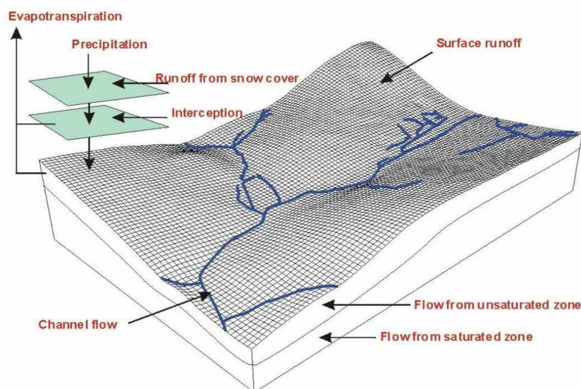
Fig. 1. General structure of a hydrological rainfall-runoff model (Jeníček, 2007).
